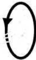
Figure 4.10. Maxwell's fourth equation: Electric fields can curl as well as diverge. Fluctuating magnetic fields produce curling electric fields (corresponding to Faraday's law).
